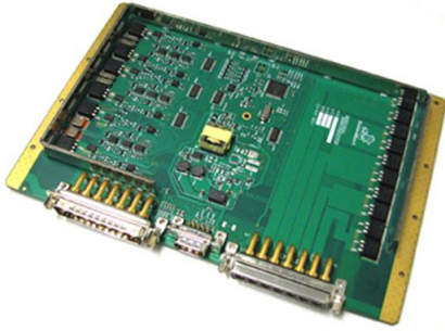
Multi-Channel Solid State Power Controller: Diamondback Series Conduction cooled card, carrying up to 210 A
